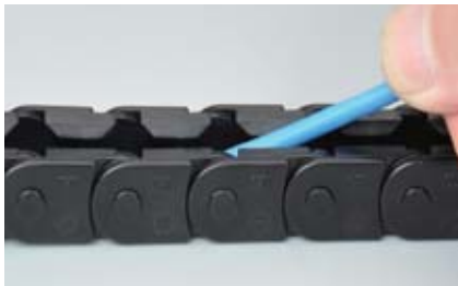
压装电缆 Press in cable
