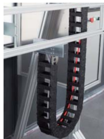
CSB-PCC® 拖链悬挂应用 Hanging applications CSB-PCC®
